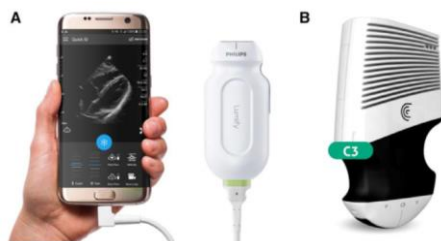
Fig. 4. Dispositivos de ecocardiografía portátiles inalámbricos, con sonda USB. (Chamsi-Pasha MA, Sengupta PP, Zoghbi WA. Handheld Echocardiography: Current State and Future Perspectives. Circulation. 2017 Nov 28;136(22):2178-2188. doi: 10.1161/CIRCULATIONAHA.117.026622.)
